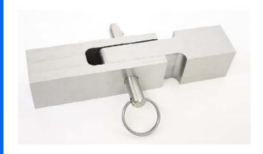
NOTE 030'-900' RADE ON HOLE EDGES TO PRIVENT MARRING THE QUICK PILLAGE PIN DURING PROOF TESTING MINOR SCRATCHES ARE ACCEPTABLE.
