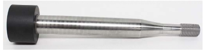
Tensile Nut Proof Load Test Fixture
