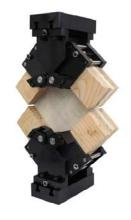
Model No. ASTM.D2719.10 Specimen Size or Difference Between Fixtures
