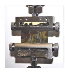
Model No.Specimen Size or Difference Between FixturesGRIP.90100.202" wide and 15 mils thick
