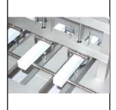
(2) 1/2" diameter supports 1/2" Loading nose Specimen Loading Bracket Alignment bearing
