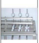
Model No. ASTM.D2990.24 - 6 Position 4-1 multiplier 100 pound Loading Flexure Creep Testing Stand for flexural creep testing in accordance with ASTM D2990 and other creep testing methods.
