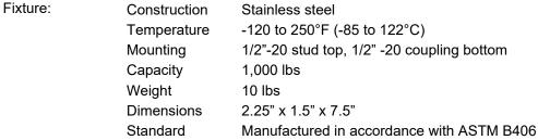
Model No. ASTM.B0406.10- Three Point Transverse Rupture Flexure Fixture for Cemented Carbides
